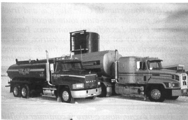
Two Cen-Alta trucks unloading salt water in the salt water disposal well
