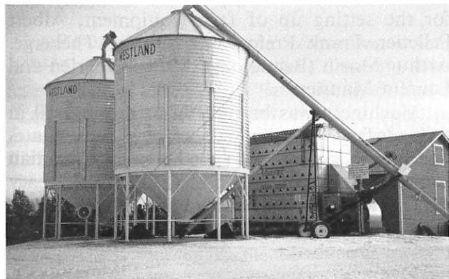
Hopper bottoms for grain bins, saving valuable time and eliminating unpleasant work
