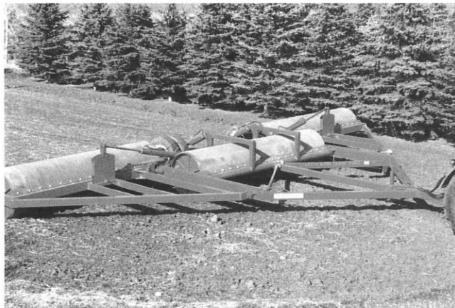
40' wide land roller built in the spring of 1992 for Joe St. Denis. He is using it to roll his fields after seeding. The objective is to flatten dirt lumps and push in stones, so when farmers harvest they will not pick up these unwanted materials, thus reducing combine wear and breakdown
