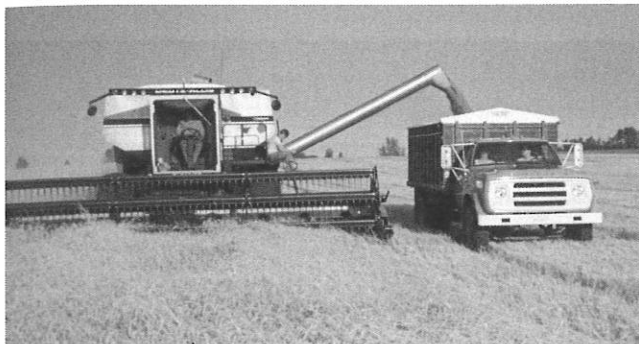
Combining and unloading on the go, N 6 Deutz-Allis combine C.B. and mobile phone. 1994 retail price - $220,000.
