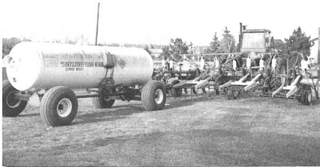
Three in one operation – chisel ploughing, harrowing and applying anhydrous ammonia, John Deere #8450 – 4 wheel drive, 240 H.P. tractor with finger tip hydraulic control, radio cassette, C.B. radio, mobile phone, plus air conditioning. 1994 retail price – $137,000; 33' chisel plow – 1994 retail price $27,000; 33' Tine harrow 1994 retail price – $2,000.
