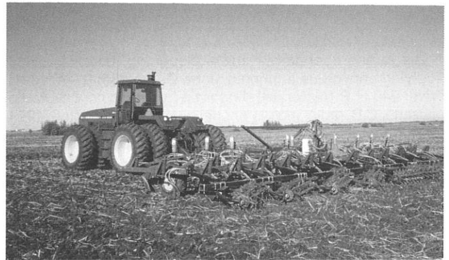
Cultivating and Harrowing, John Deere 4 wheel drive tractor #8760-300 H.P. with C.B., mobile phone and air condition, 39 foot chisel plow & active harrows. 1994 prices: tractor $165,000, chisel plow $30,000, active harrows $7200.00
