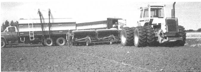
Seeding wheat and alfalfa and applying fertilizer all in one operation with a 32-foot John Deere Hoe Drill pulled by a 2670 Case tractor. The drill is filled by hydraulic augers from the Drill Fill. Approximate values: tractor ($65,000), drill ($30,000), trucks ($28,000 each), drill fill ($4,000)
