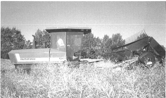
Swathing canola with self-propelled Westward Swather – 25' table. 1994 retail price $65,000.
