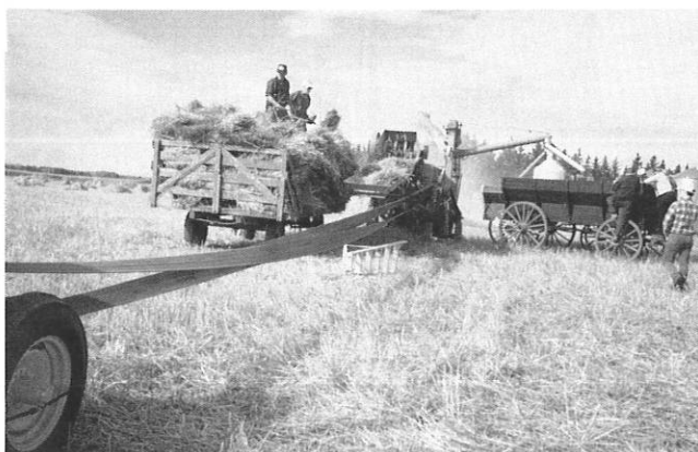
Feeding the restored McCormick Deering 28" thresher driven by a restored John Deere D tractor.
